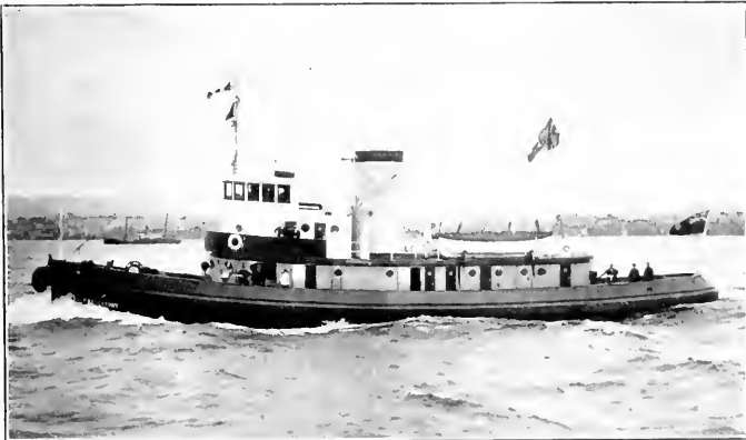
Diesel-electric tug Prescott which is arranged for remote control from the bridge or from the tow.
